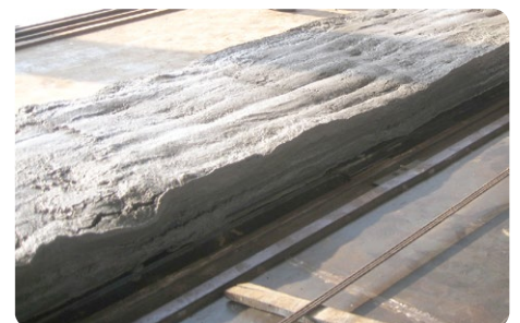
Figure 2: An example of collapsing Hollowcore concrete due to incorrect consistency
