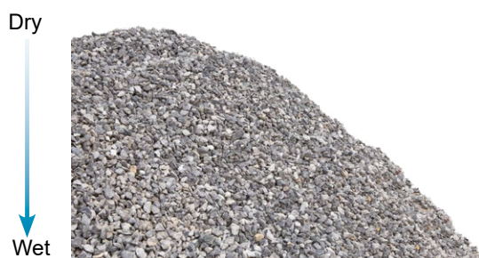
Figure 1: Natural Moisture Drainage through an Aggregate Stockpile
