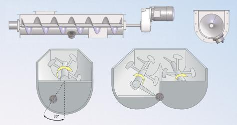
The Hydro-Mix XT can be mounted in many different locations where there is a continuous flow of material across the ceramic faceplate. These include drying, ducting, conveying and mixing systems.
