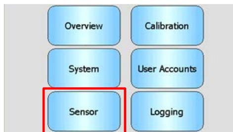
When the Sensor button on the Main Menu is touched, a list of the connected sensors appears (only if more than one is connected). Select the required sensor to access the Sensor Setup screens (Figure 22).
