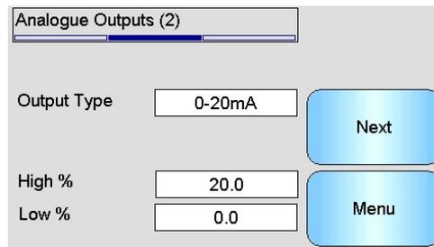
Figure 27: Analogue Outputs Screen 2
