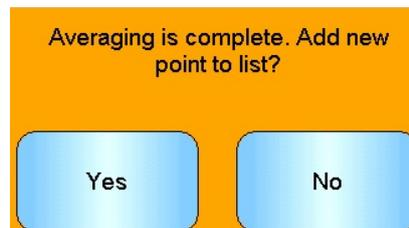
If manual averaging is to be used ensure that the averaging is only started once the material is flowing and is stopped when the gate is closed or the flow stops.
