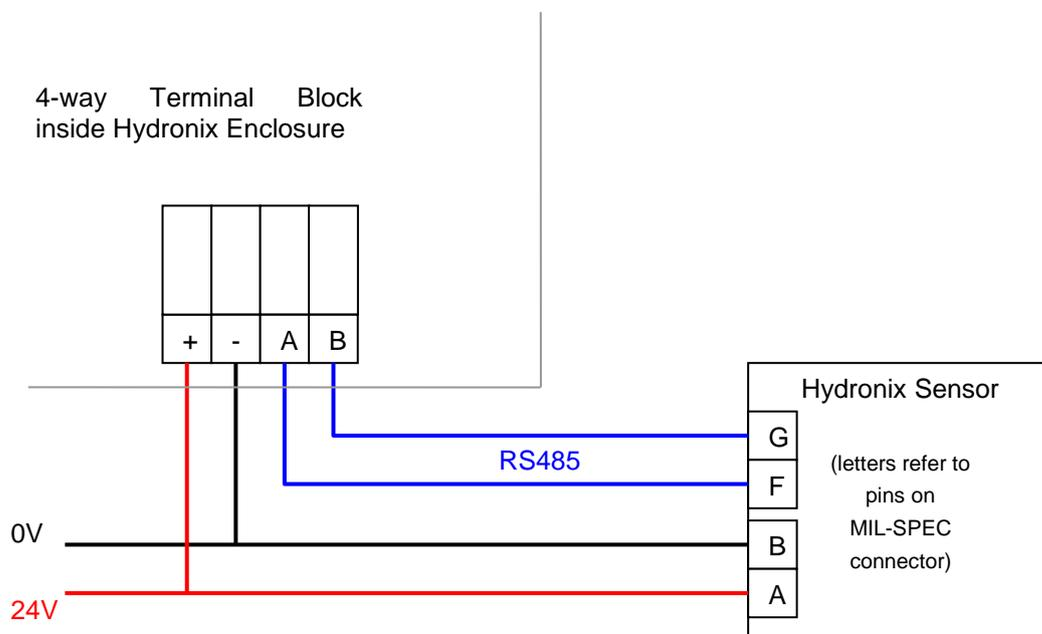
Figure 7: Hydro-View Wiring Diagram (with Hydronix Enclosure)
