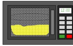
18. Carefully break up any lumps of material using a metal spoon. Do not allow any material to be lost from the bowl or to stick to the spoon. Only break up lumps once the material surface is dry.
