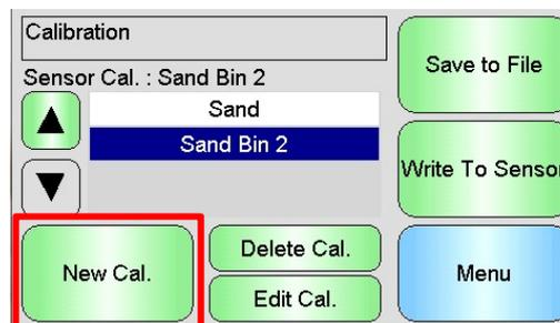
3. Enter a calibration name and configure the Calibration Type, Tolerance, Measurement Mode (if available) and Quick Start Rules (if applicable).
