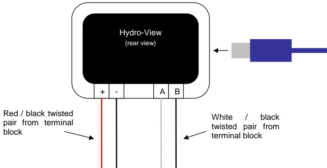
**Figure 8: Hydronix Enclosure Internal Wiring**
