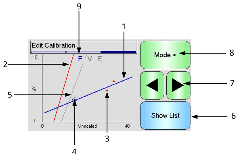
Figure 54: Edit Calibration Points Graph Screen
