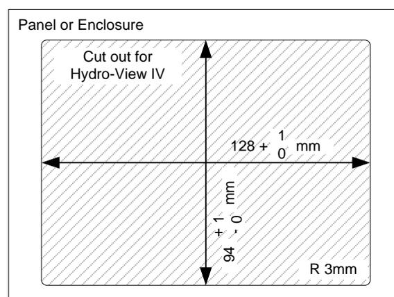
**Figure 4: The Panel Cut-Out for the Hydro-View**
