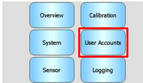
The User Accounts Screen allows users to 'log in' to the Hydro-View with different permissions levels. After completing operations as Supervisor or Engineer it is advisable to log out to prevent inadvertent access and changes to the system setup. It is necessary to log out as one user before logging in as a different user. By default the permissions are set to Plant Operator.
