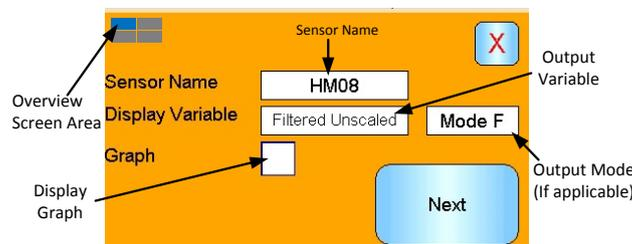
Figure 19: Overview Screen Sensor Selector
