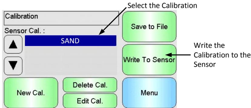
Figure 80: Write Calibration to the Sensor
