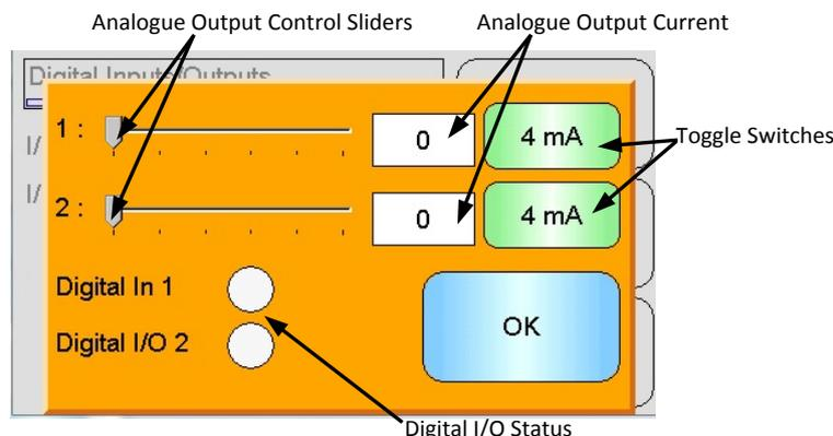
**Figure 29: I/O Test Screen**
