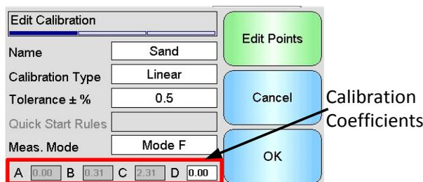
**Figure 73: Calibration Coefficients**
