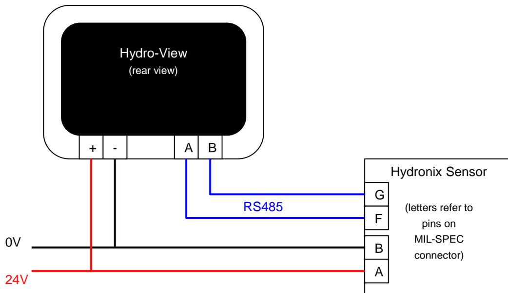
Figure 6: Hydro-View Wiring Diagram
