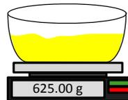
20. Continue to re-heat and weigh the material until the weight remains constant between two heating cycles. This indicates that the material is fully dry.
