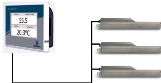
Although it may appear simpler, wiring in a star configuration with each sensor wired back to the Hydro-View should be avoided.
